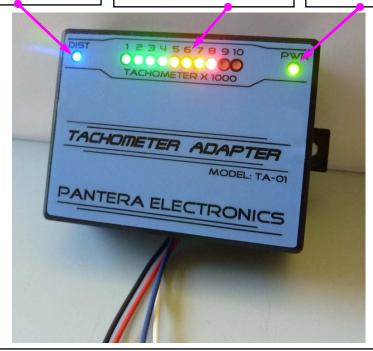
RED wire - connect to +12V when the ignition switch in the "Ignition" position.
