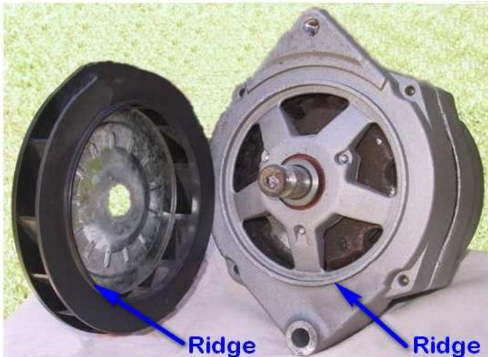
The photo below shows a model Si Delco alternator, viewed from the rear. When viewed from the rear, the air intake area is the most distinguishing visible feature of the Si.
