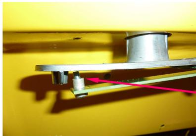
Use the factory mounting screws to assemble the LED License Plate Light board with the light bulb socket bracket and mount to the body. Use the spacers between the LED board and the factory bracket.
