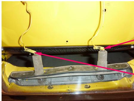
Lower the light bulb socket bracket and disconnect the wires to the light bulb sockets.
