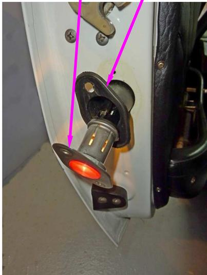
Grasp the lens flange and pull the incandescent bulb socket from the lens flange.
