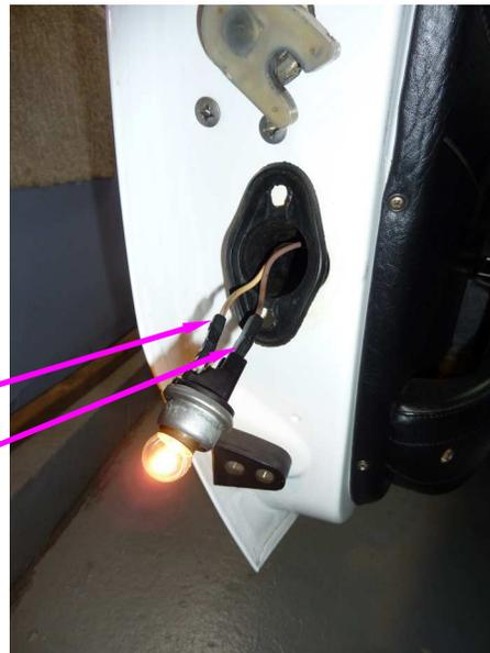
It does not matter which order to install the Door Jamb LED board in the lens flange or connect to the wires to the Door Jamb LED board and then install in the lens flange. See page 4.
