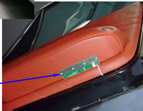
The wires can be wrapped around the edge of the door panel. Then painted black or the color of the door panel with a marker pen.
