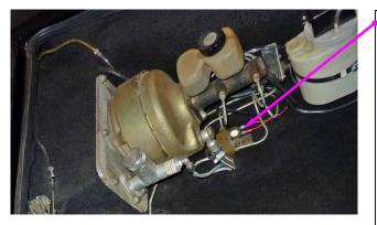
There are 2 RED wires that connect to the factory hydraulic brake switch in the trunk. These are disconnected and pulled back through the grommet in the bulkhead. The terminals may need to be cutoff and sleeves removed. Leave the PVC sheathing on the wires.
