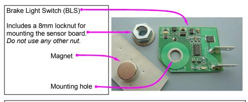
The BLS can drive the factory incandescent lamps or modern LED lamps or a combination. The BLS can supply 8 amps constant current.
