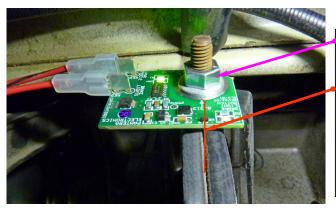
Slide the BLS onto the stud and install the nut.
