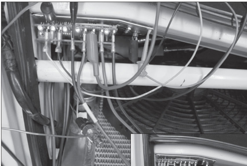
Above and right: On-board indicators for power on, delay timer complete, maximum fan speed and power from each output to the fans. All connections and indicators are arranged at the top of the controller board for easy access.
