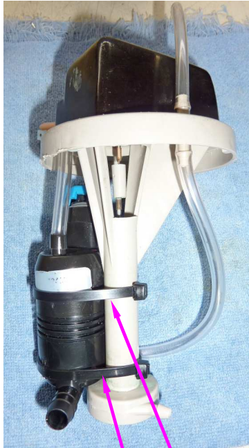
Simple tie-rap mounting
