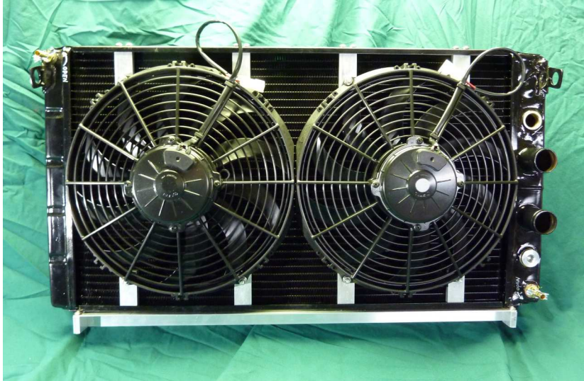
The Spal fans are mounted on the factory modified radiator to Pantera Electronics specifications and PE design mounting brackets.
