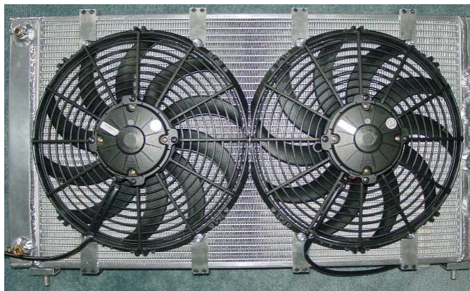
The Spal fans are mounted on the Fluidyne Radiator with PE design brackets.
