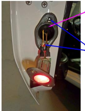
Insert the lens flange and Door Jamb LED assembly into the boot feeding the wires back through the hole in the end of the boot.
