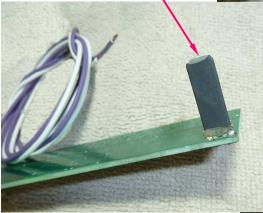
The wires can be wrapped around the edge of the door panel. Then painted black or the color of the door panel with a marker pen.
