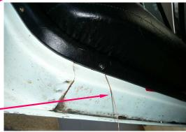
→ Tape the fish wire to the Door Courtesy wires.
