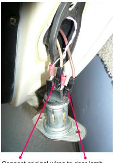
Connect original wires to door jamb light socket tabs.
