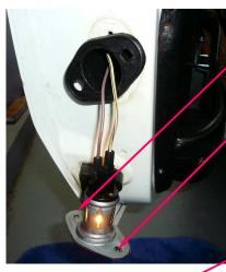
Remove (2) screws that mount the door jamb light.
